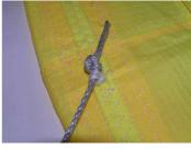
Creating a channel for the fid using a Samson splicing tool, (a long skinny nail would work).
